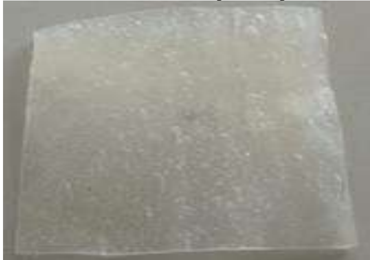
Figure 1. The bioplastic obtained by employing ingredients 50 grams of cassava starch, 25 ml of glycerol, 25 ml of acetic acid (vinegar), 50 ml of water, and 25 ml of ethanol
